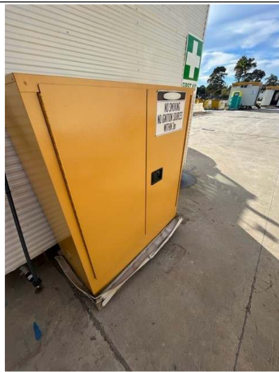
Photos 6 & 7: Jerry cans of ULP and diesel were stored inside a purpose-built container. The container required labelling in accordance with the GHS
